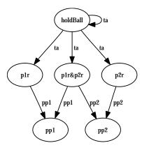
Figure 2: Creation of the SNMDP. The original node with the action *holdBall* is split creating nodes to represent the conditions
